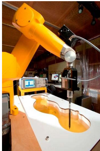
Figure 3-2 DASY4 SAR Measurement System
