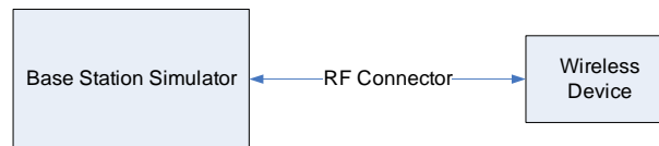
Figure 15-1 Power Measurement Setup
