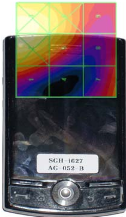
Figure 17-4 E-Field WD Scan overlay
