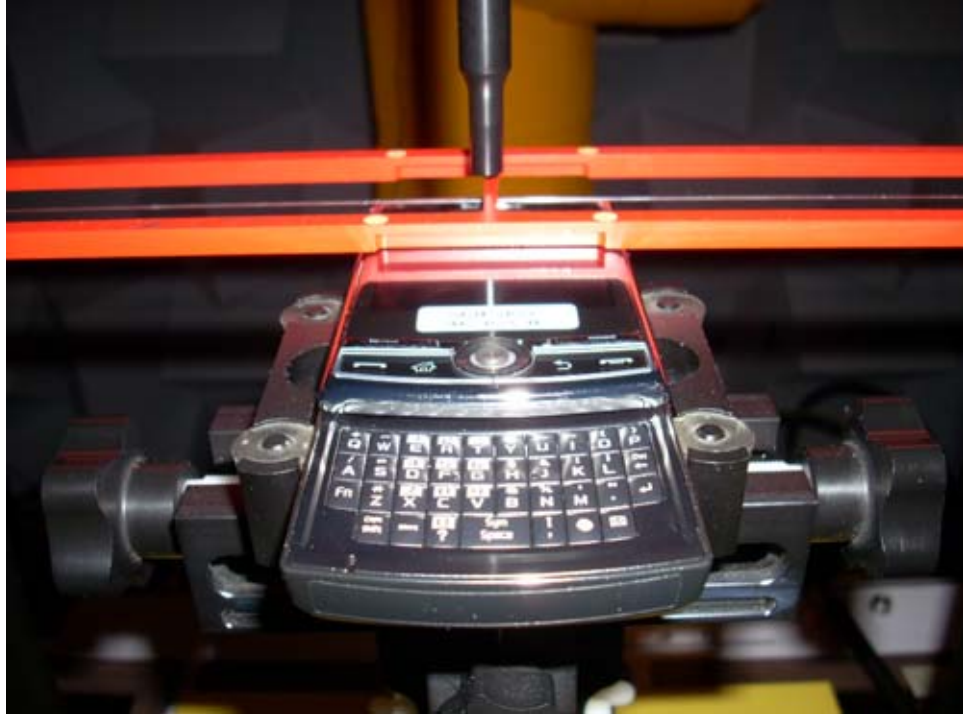
Figure 17-1 Ear Reference Point HAC Phantom Alignment
