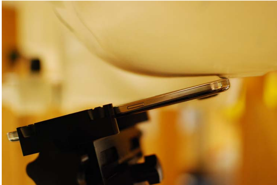
SAR Test Setup Photo 4 - Left Tilt
