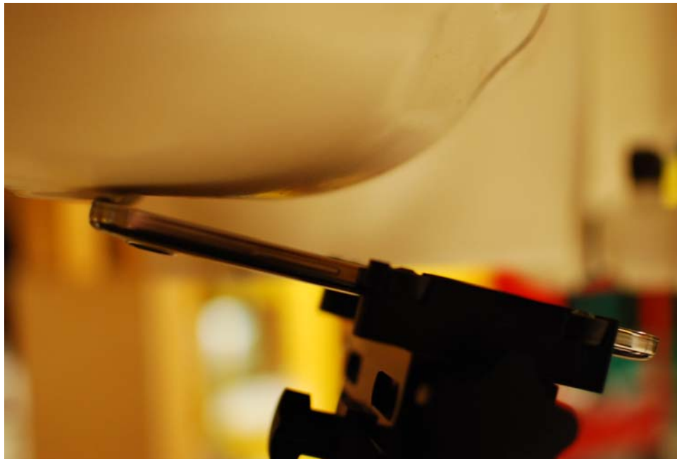
SAR Test Setup Photo 2 - Right Tilt
