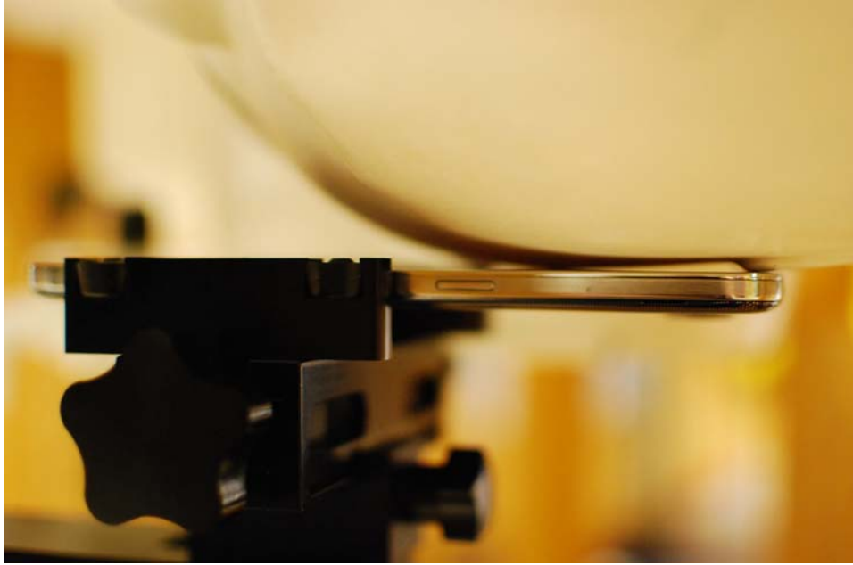
SAR Test Setup Photo 3 - Left Cheek
