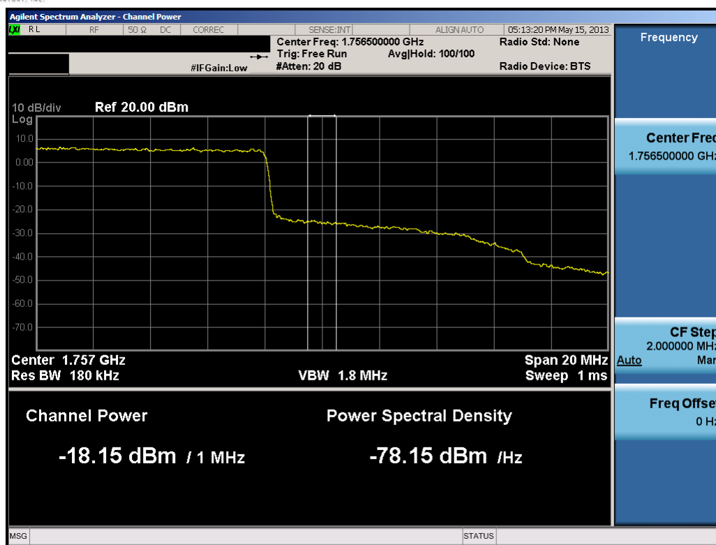
Plot 9-26. Upper Extended Band Edge Plot (10.0MHz QPSK – RB Size 50)
