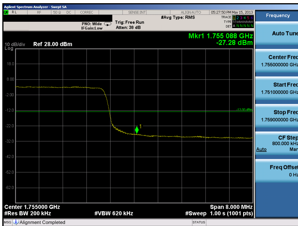
Plot 9-53. Upper Band Edge Plot (20.0MHz QPSK – RB Size 100)
