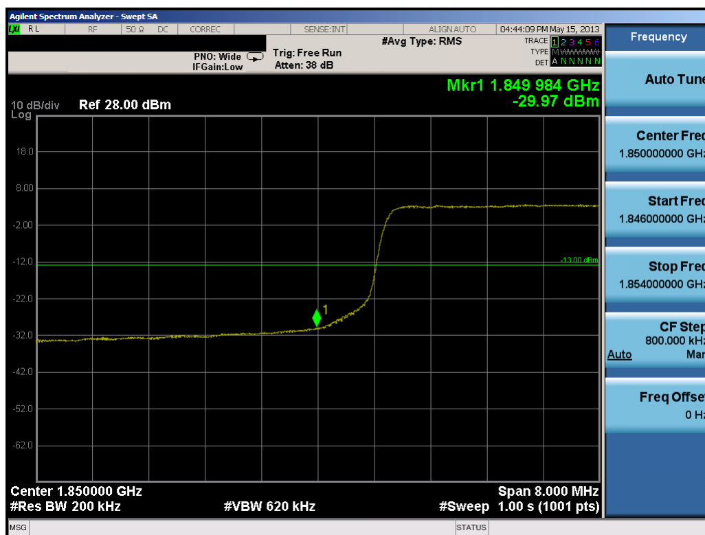
Plot 10-43. Lower Band Edge Plot (20.0MHz QPSK – RB Size 100)
