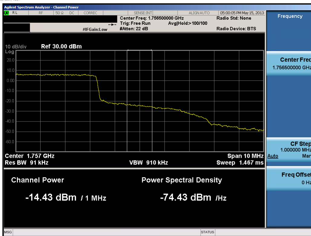
Plot 9-12. Upper Extended Band Edge Plot (5.0MHz QPSK – RB Size 25)
