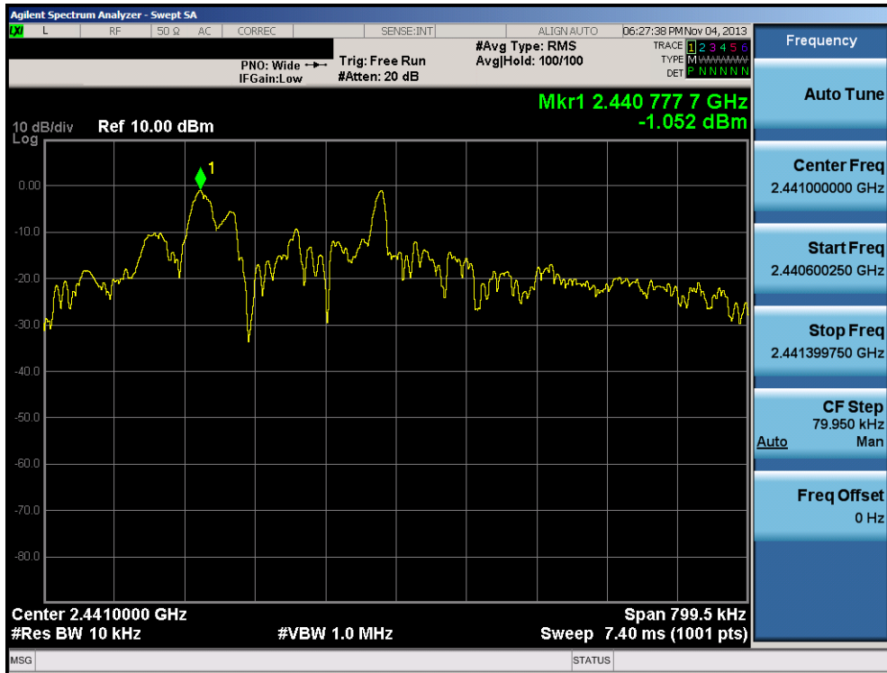
Plot 6-8. Power Spectral Density Plot (2441MHz – Mid Channel)
