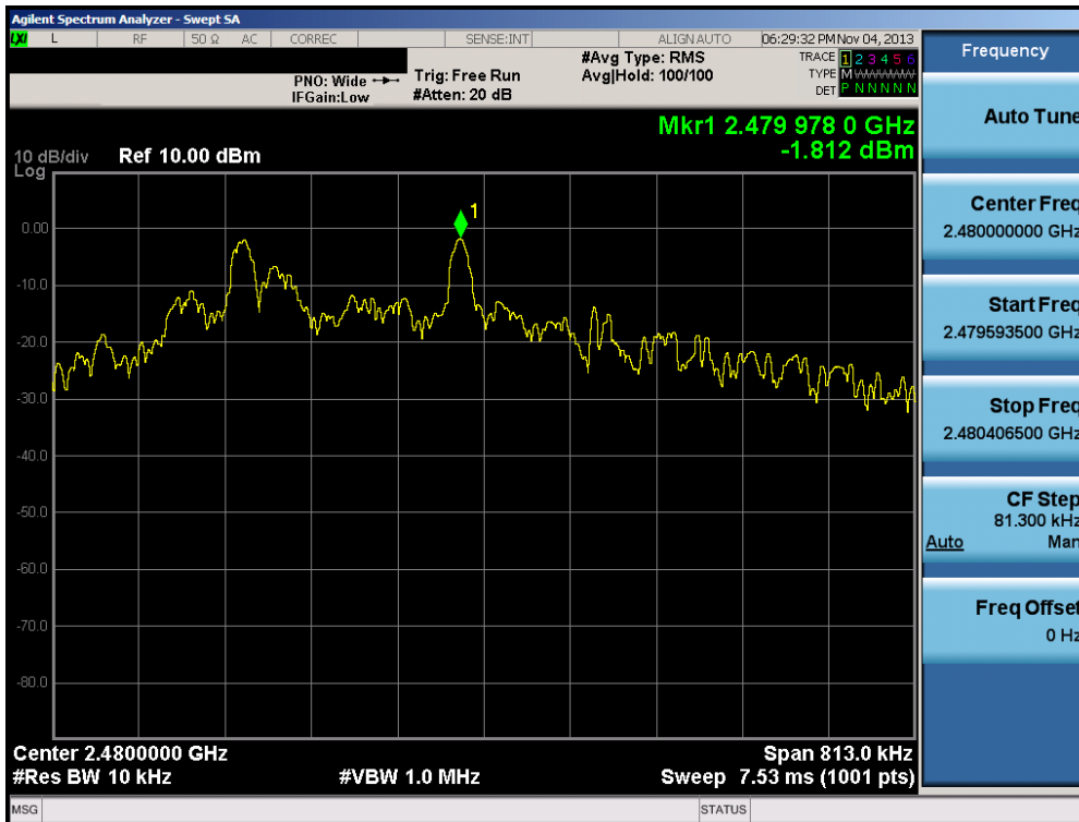
Plot 6-9. Power Spectral Density Plot (2480MHz – High Channel)
