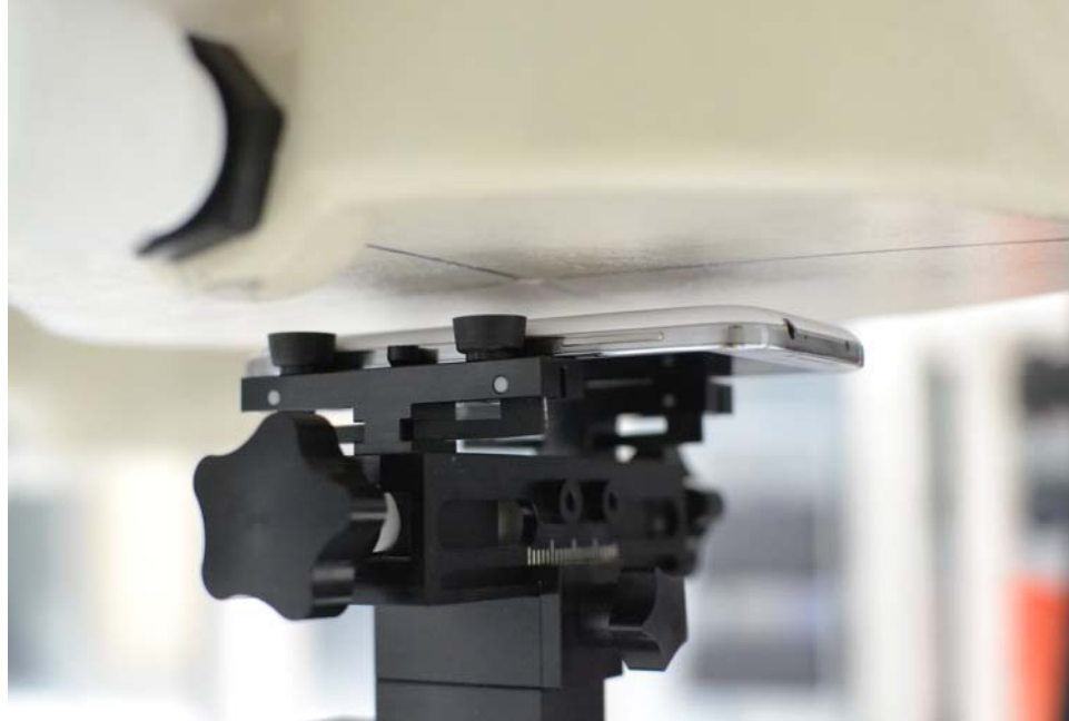
SAR Test Setup Photo 6 – Back side at 1.0 cm with Wireless Charging Cover
