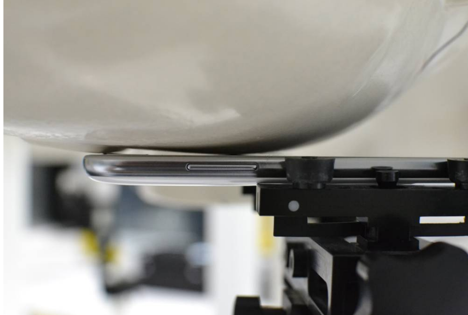
SAR Test Setup Photo 1 – Right Cheek
