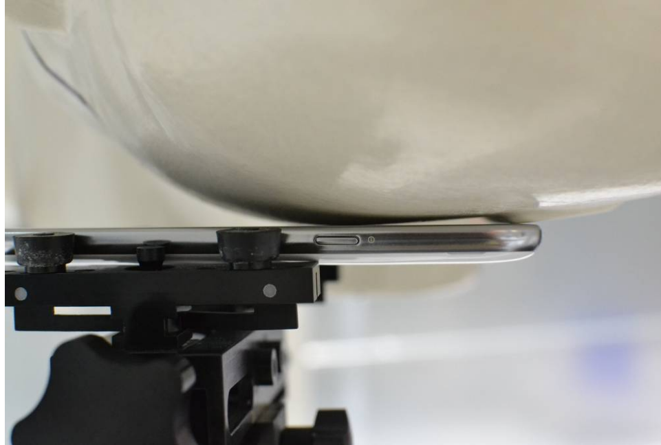
SAR Test Setup Photo 3 – Left Cheek
