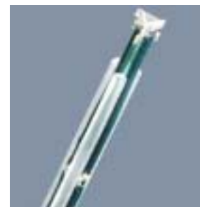
Figure 3.4 Probe Thick-Film Technique
