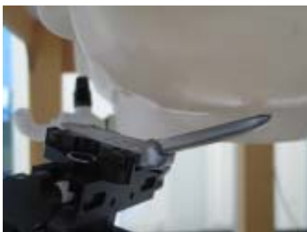
Figure 8.3 Right Head SAR Test Setup -- Ear/Tilt 15° Position--
