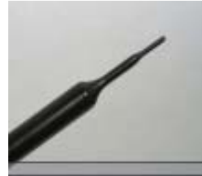
Figure 3.4 Probe Thick-Film Technique
