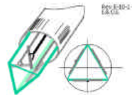
Figure 4-2 Triangular Probe Configuration
