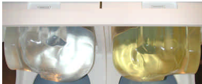
Figure 8-1 Left and Right SAM Phantom shells
