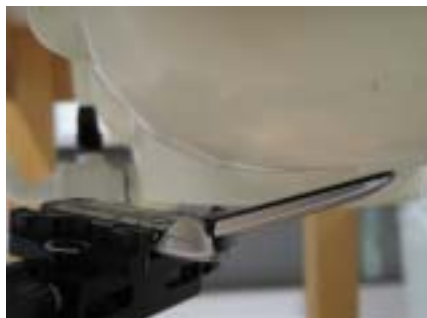
Figure 8.3 Right Head SAR Test Setup -- Ear/Tilt 15° Position--
