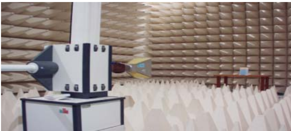
Figure2. Photograph of 3m Fully Anechoic Chamber
