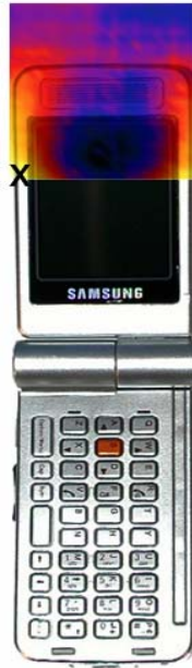
Figure 27 Sample E-field Scan Overlay
