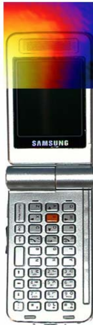
Figure 28 Sample H-field Scan Overlay
