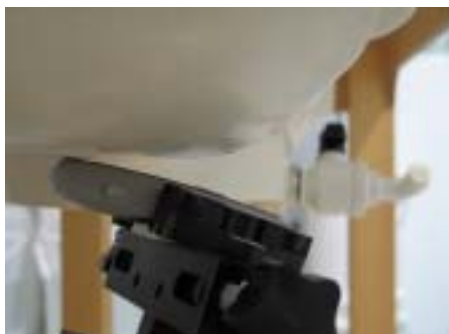
Figure 8.7 Right Head SAR Test Setup -- Ear/Tilt 15° Position--
