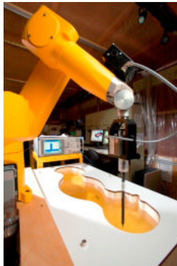
Figure 3-2 DASY4 SAR Measurement System
