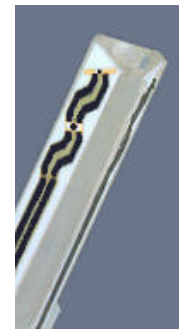
Figure 4-2 Probe Thick Film Technique
