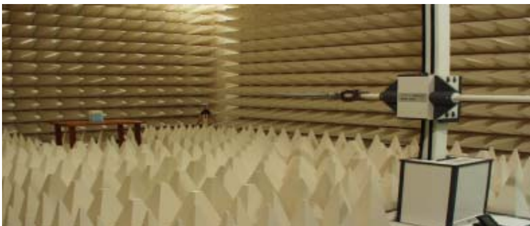
Figure2. Photograph of 3m Fully-Anechoic Chamber
