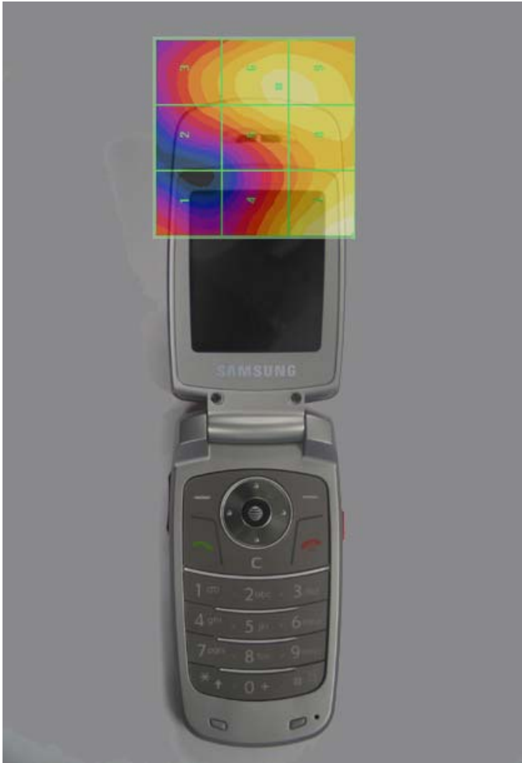
scan overlay with actual device(E-field)
