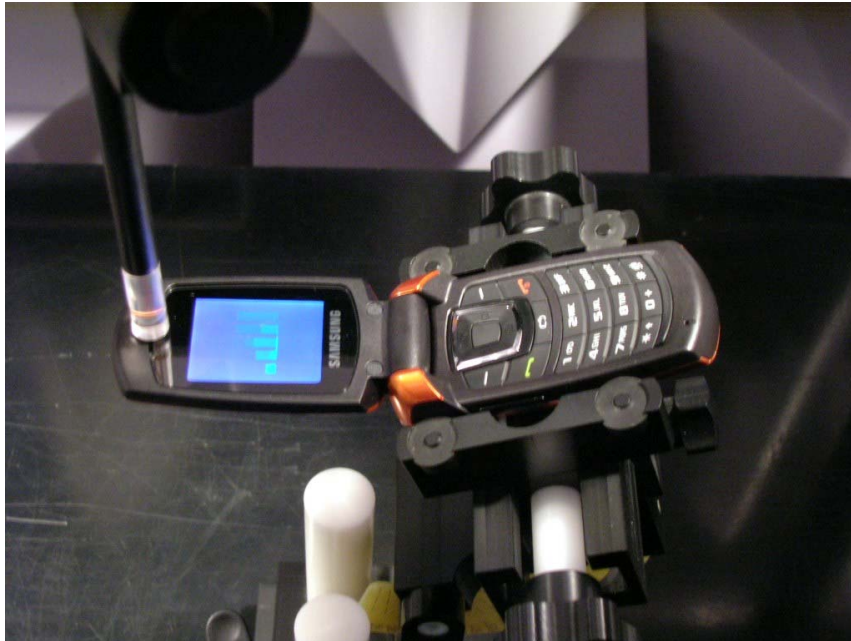
Figure 12-1 Test Setup for Wireless Device
