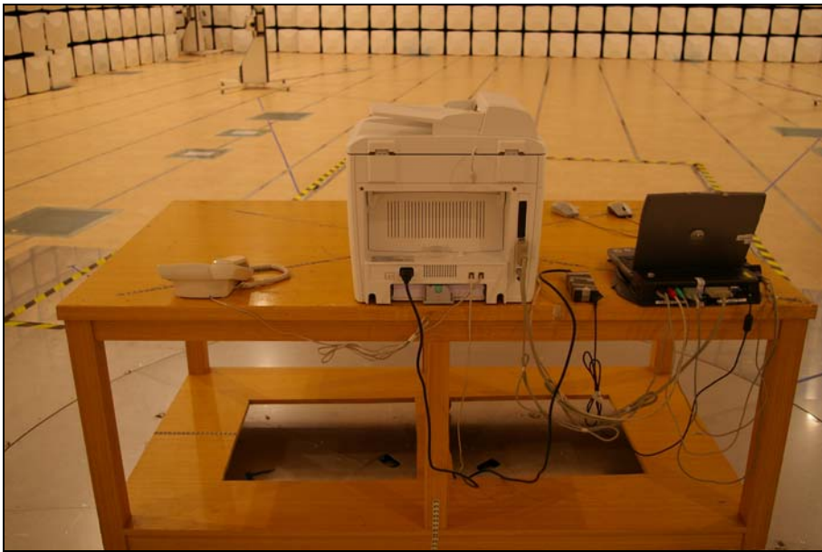
Picture 4. Radiated emission (Rear)
