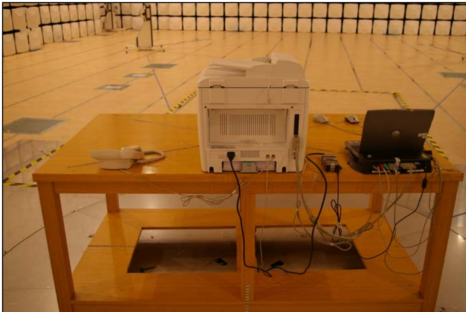
Picture 4. Radiated emission (Rear)
