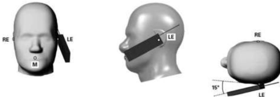
Figure 6.5. Tilt 15° position of the wireless device
