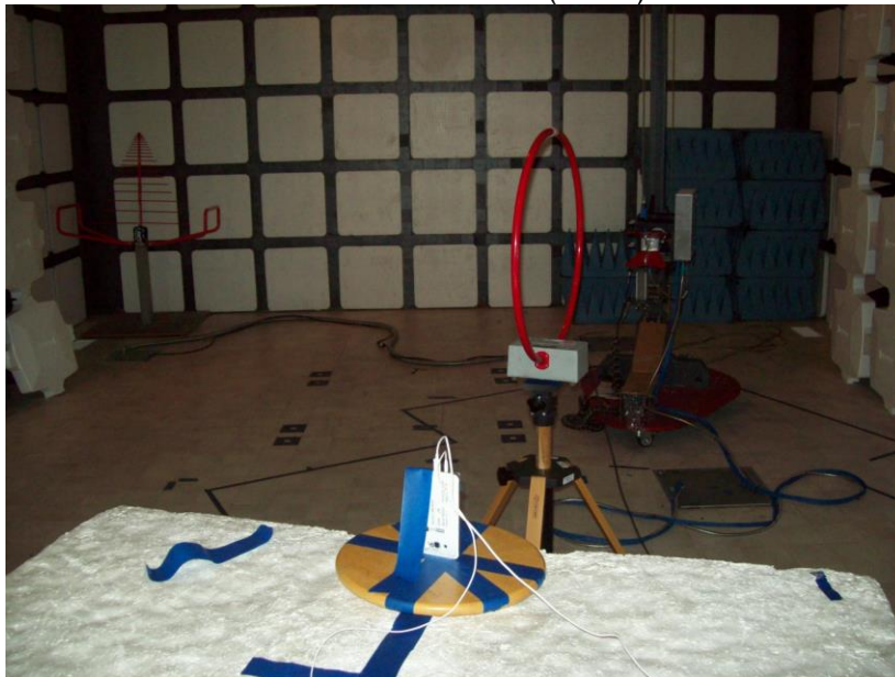
RADIATED EMISSIONS BELOW 30MHz (BACK)
