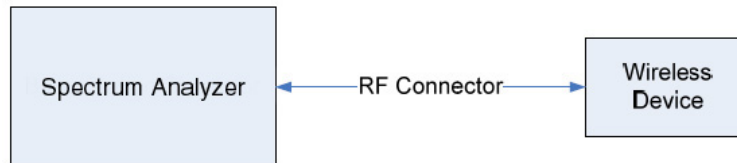
Figure 6-1. Test Instrument & Measurement Setup
