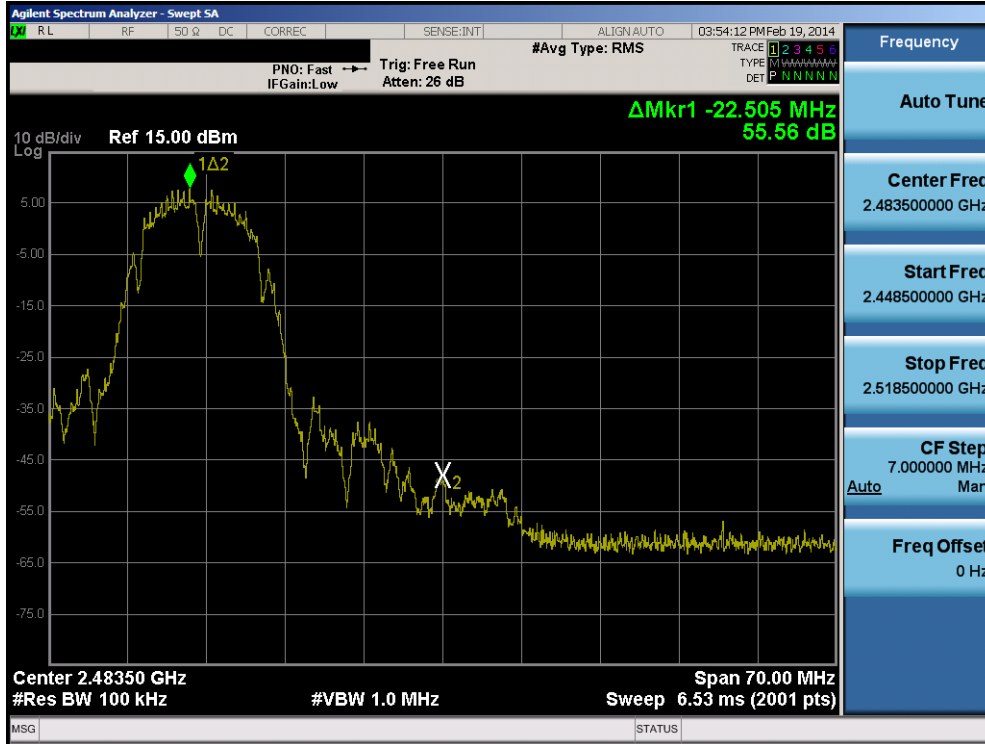
Plot 6-88. Band Edge Plot (802.11b – Ch. 11)
