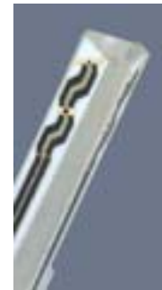
Figure 3.4 Probe Thick-Film Technique
