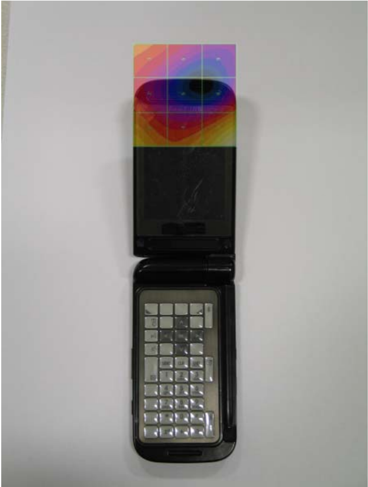
Scan overlay with actual device for CDMA (H-field)
