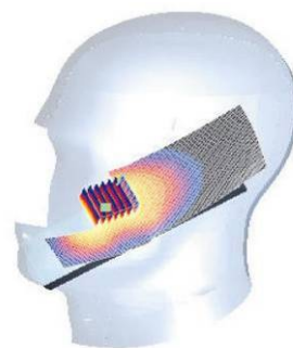
Figure 7-1 Sample SAR Area Scan
