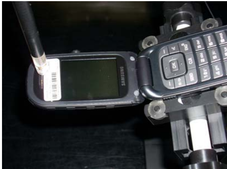
Figure 13-2 Test Setup for Wireless Device
