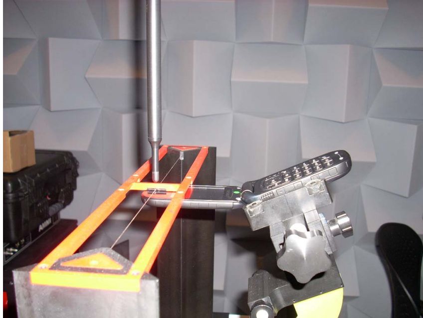
Figure 17-1 Ear Reference Point HAC Phantom Alignment
