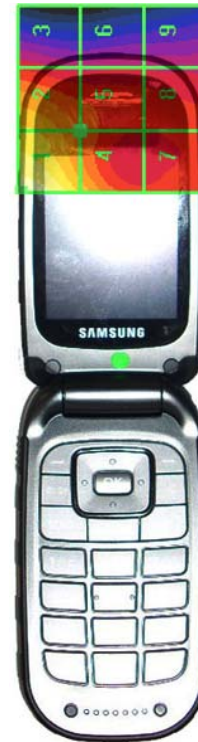
Figure 17-5 H-Field WD Scan overlay
