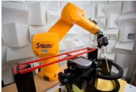
Figure 5-5 SPEAG Robotic System
