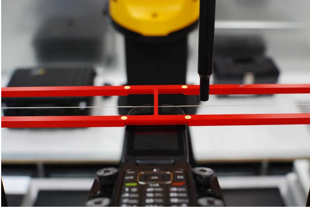
Figure 17-1 Ear Reference Point HAC Phantom Alignment
