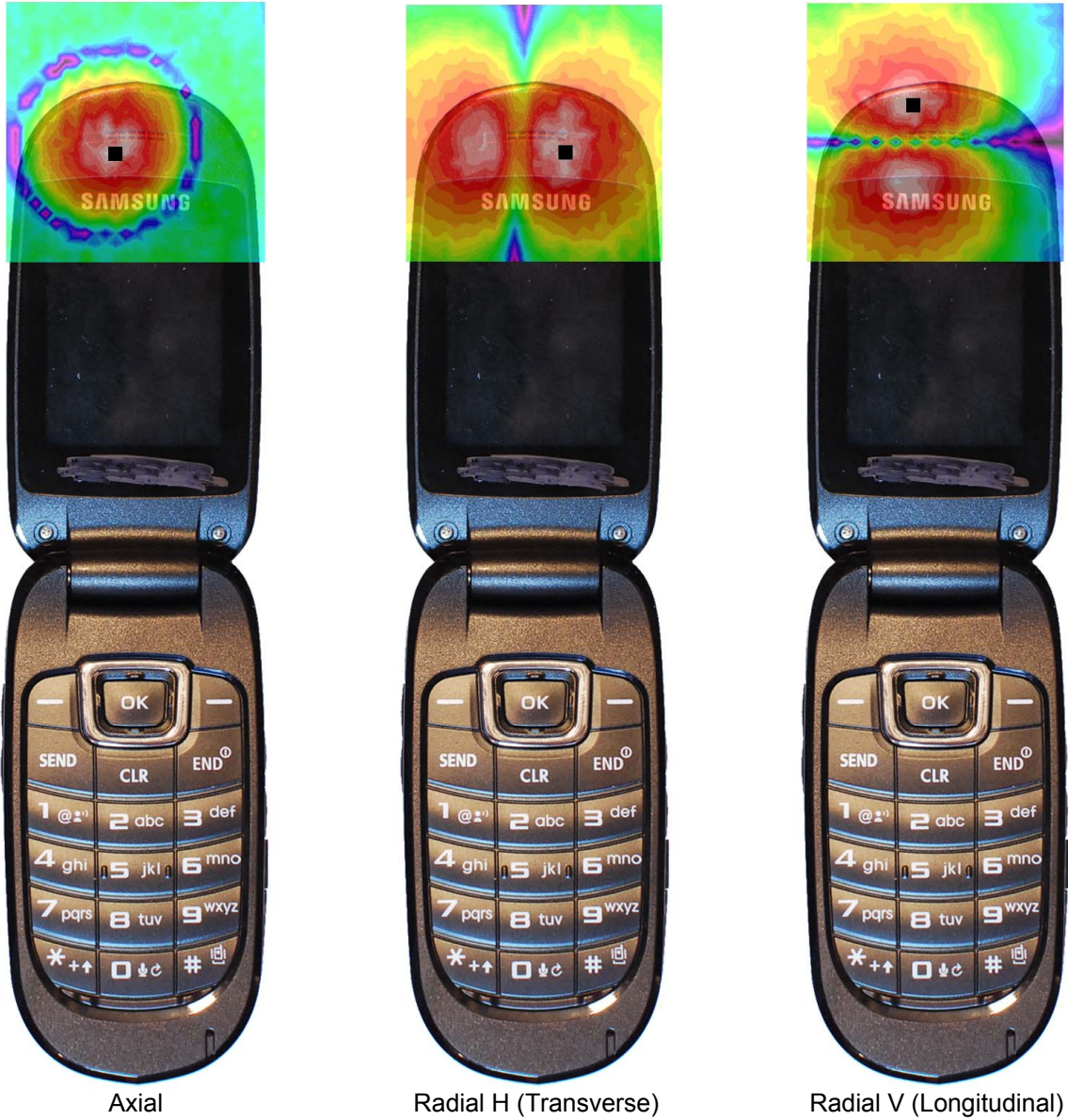
Figure 13-3 T-Coil Scan Overlay Magnetic Field Distributions
