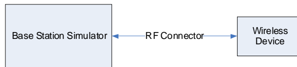
Figure 14-1 Power Measurement Setup
