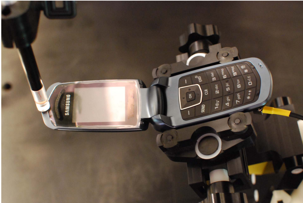
Figure 13-2 Test Setup for Wireless Device
