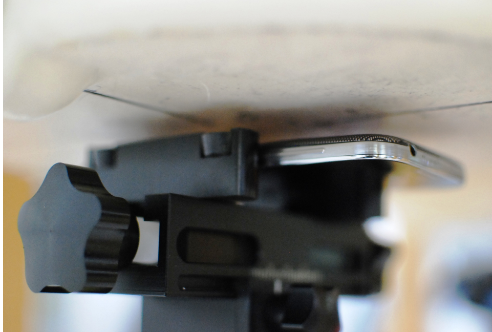
SAR Test Setup Photo 1: Back Side at 1.0 cm with Standard Battery Cover
