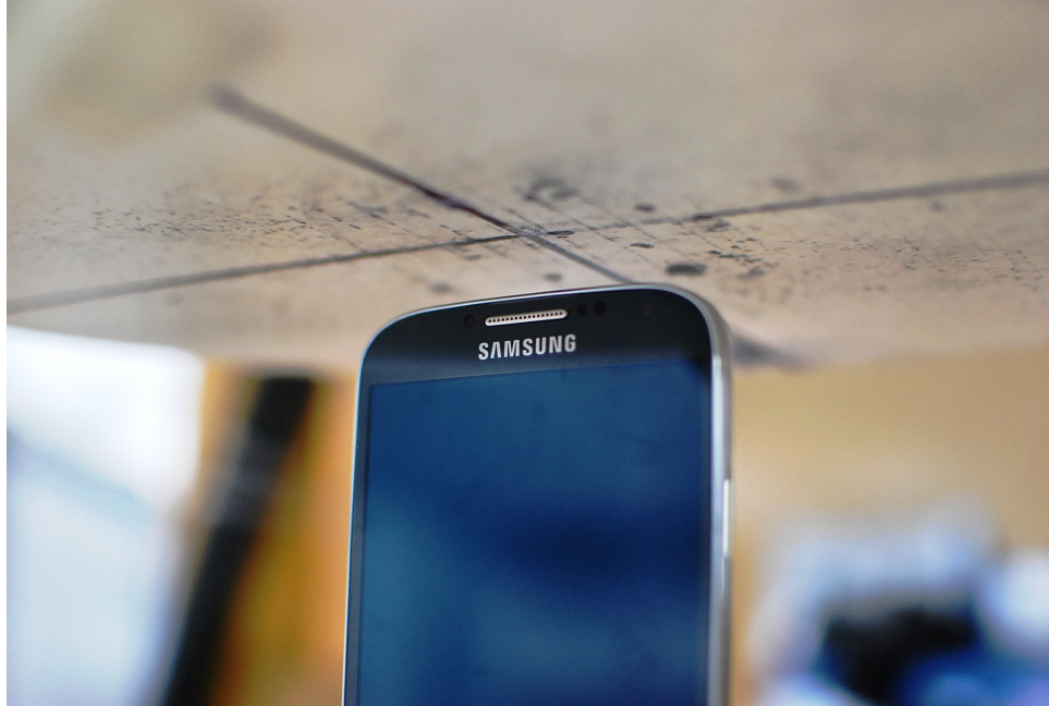
SAR Test Setup Photo 3: Top Edge at 1.0 cm with Standard Battery Cover
