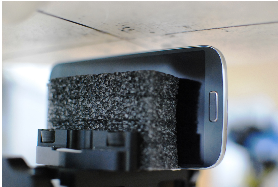
SAR Test Setup Photo 4: Right Edge at 1.0 cm with Standard Battery Cover
