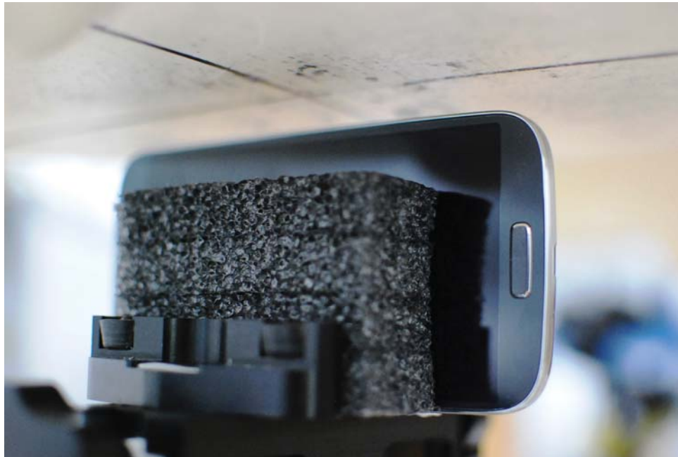
SAR Test Setup Photo 12: Right Edge with Standard Battery Cover
