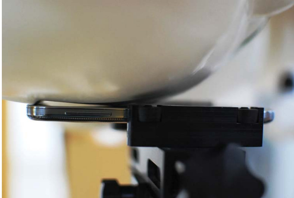
SAR Test Setup Photo 1: Right Cheek with Standard Battery Cover
