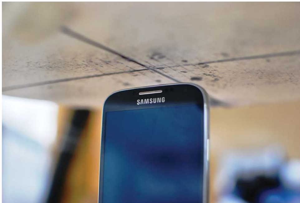
SAR Test Setup Photo 10: Top Edge with Standard Battery Cover
