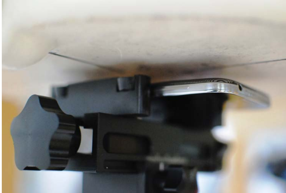
SAR Test Setup Photo 7: Back Side with Standard Battery Cover
