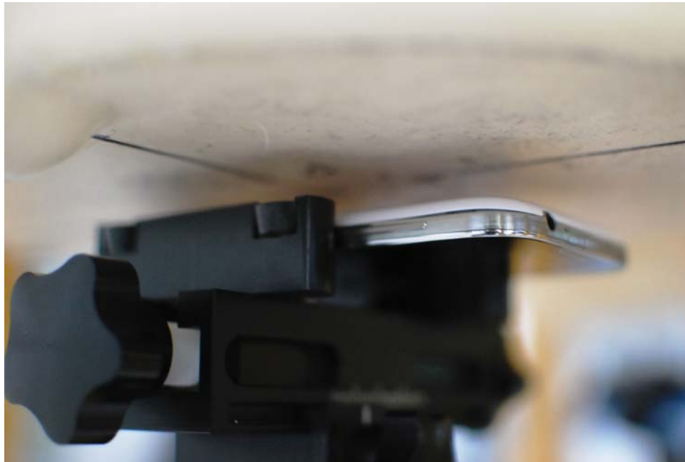
SAR Test Setup Photo 8: Back Side with Wireless Charging Cover
