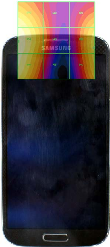
Figure 17-4 E-Field WD Scan overlay
