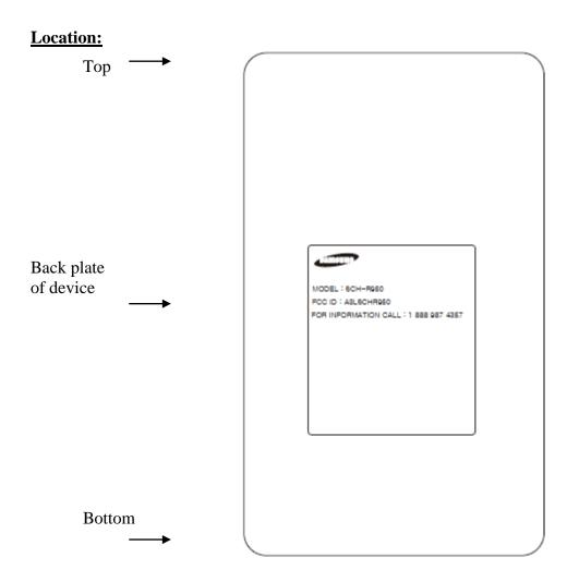
Phone: Label is placed inside of the battery compartment.
