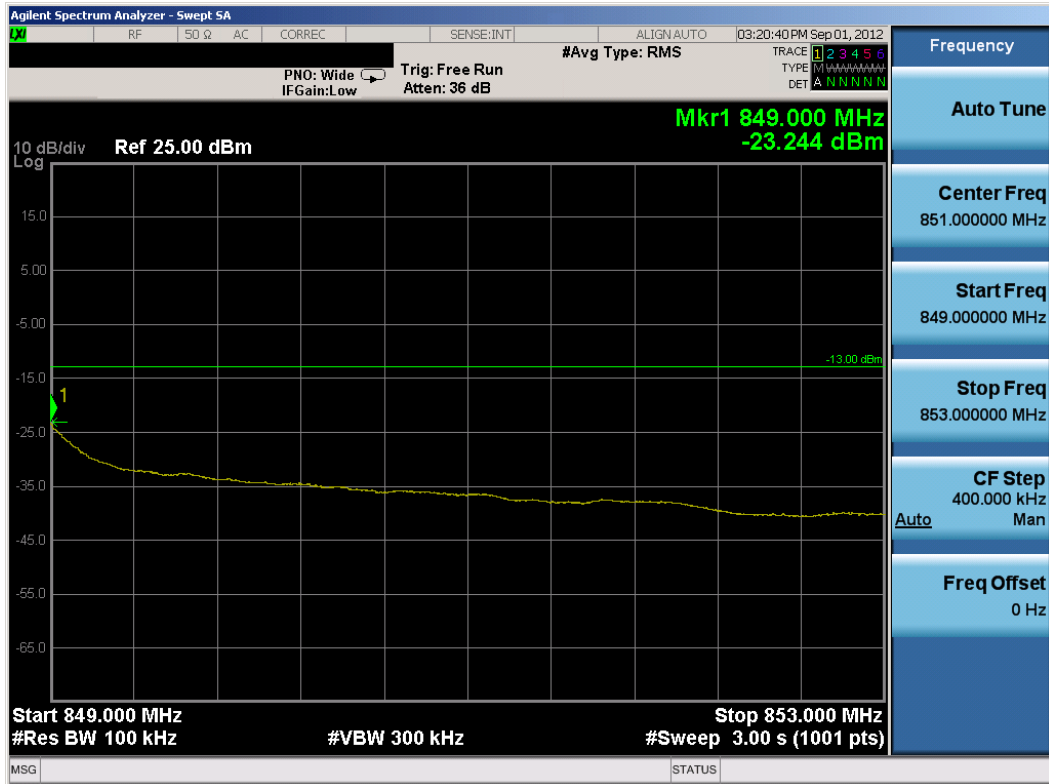
Plot 8-17. Upper Extended Band Edge Plot (5MHz QPSK – RB Size 25)
