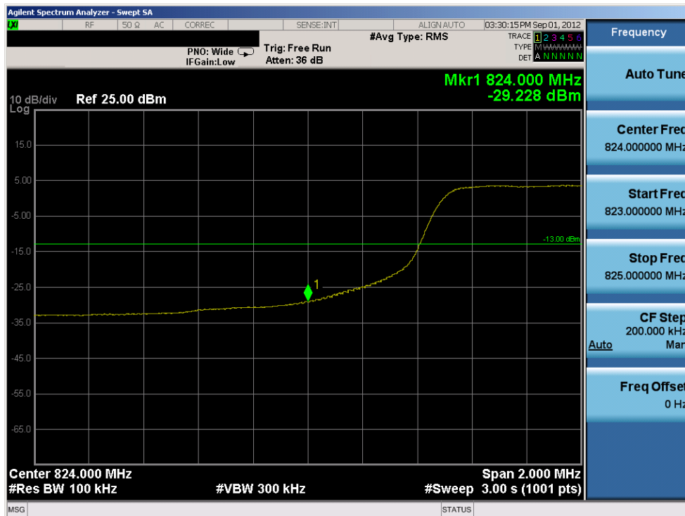
Plot 8-2. Lower Band Edge Plot (10MHz QPSK – RB Size 50)
