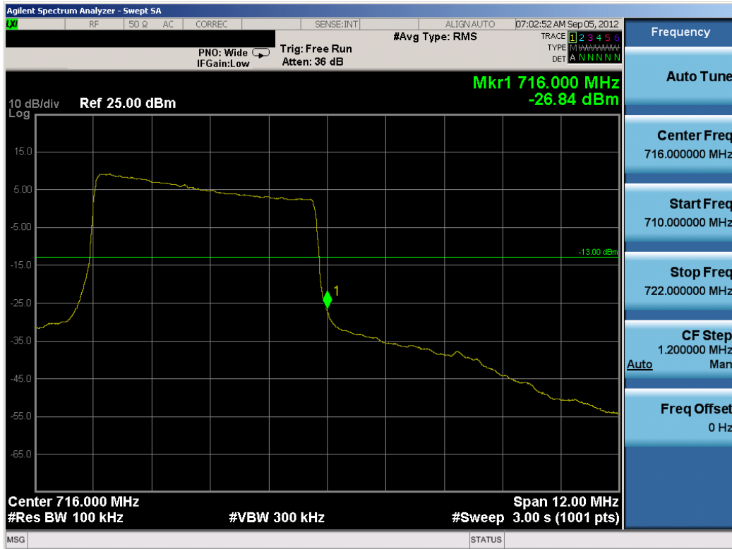
Plot 7-13. Upper Band Edge Plot (5MHz QPSK – RB Size 25)
