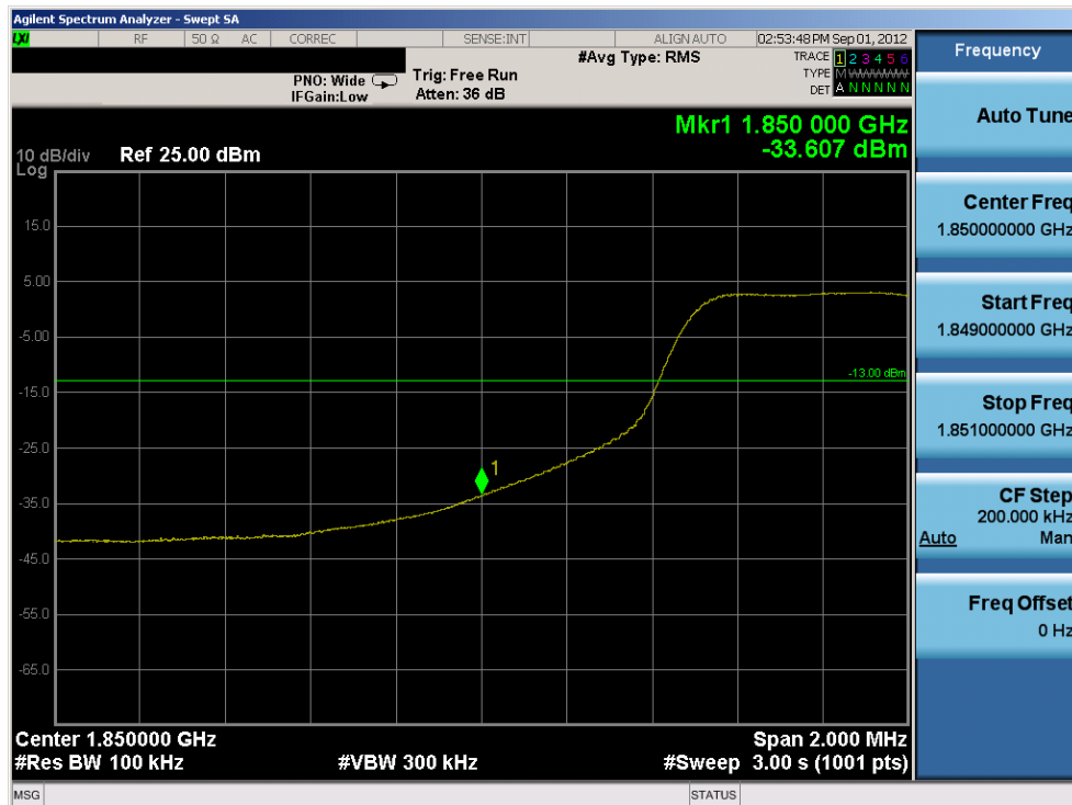
Plot 10-2. Lower Band Edge Plot (10MHz QPSK – RB Size 50)
