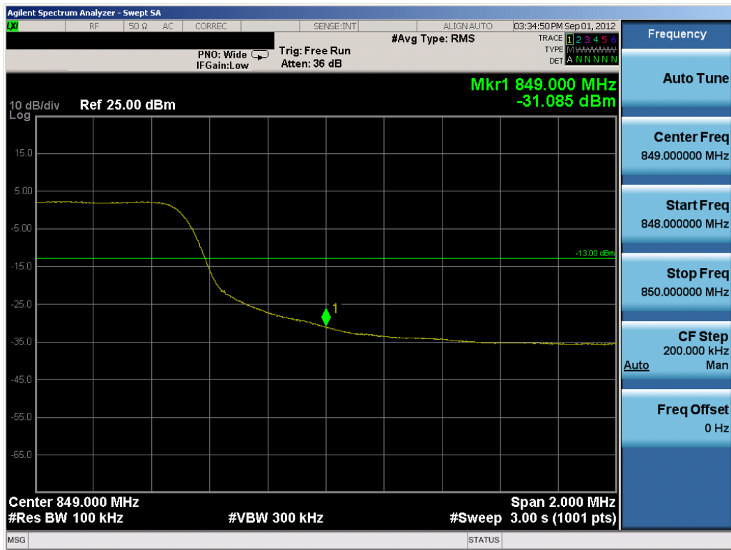
Plot 8-16. Upper Band Edge Plot (10MHz QPSK – RB Size 50)
