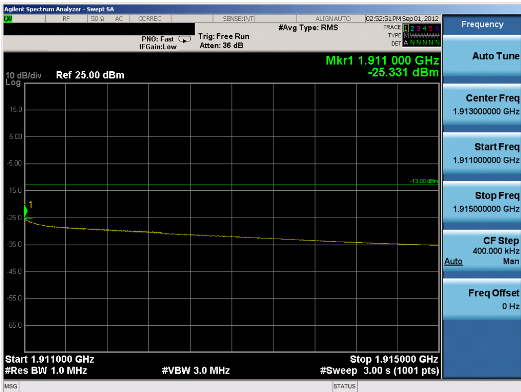
Plot 10-18. Upper Extended Band Edge Plot (10MHz QPSK – RB Size 50)
