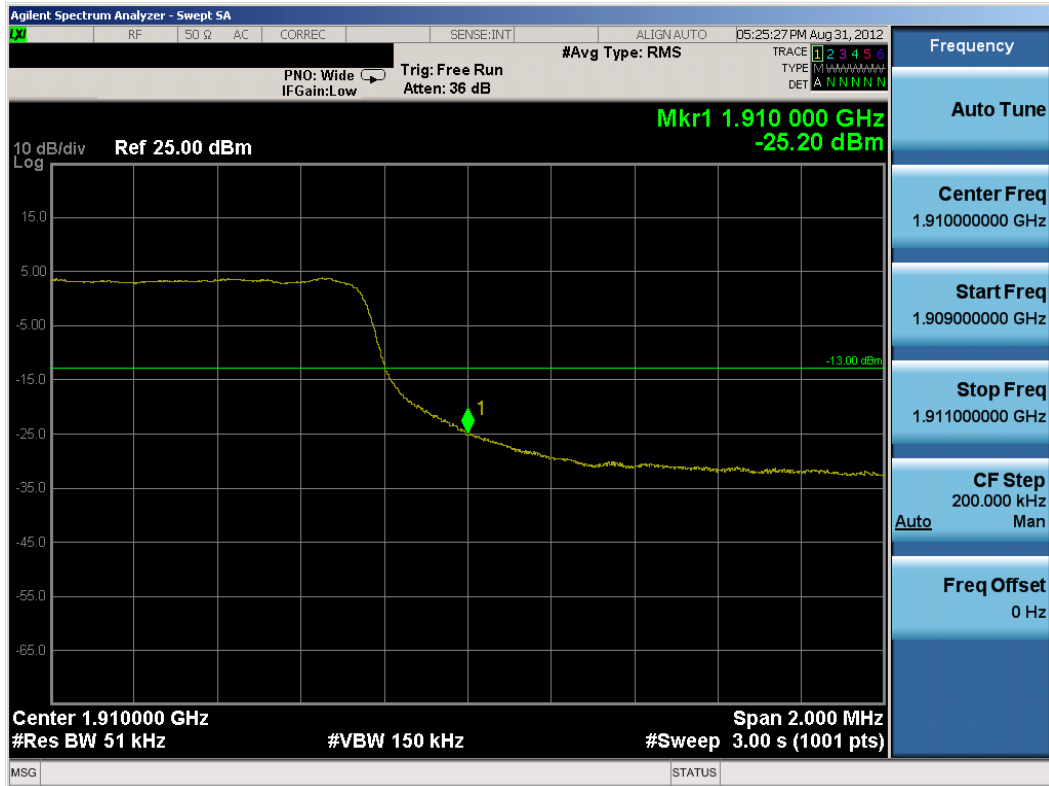
Plot 10-15. Upper Band Edge Plot (5MHz QPSK – RB Size 25)
