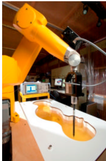
Figure 3-2 DASY4 SAR Measurement System
