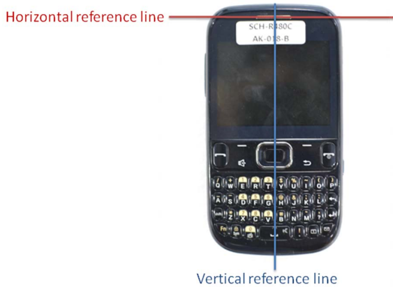
SAR Test Setup Photo 6: DUT Vertical and Horizontal Reference Lines
