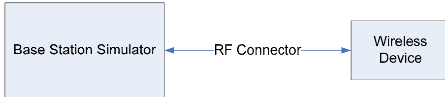
Figure 9-1 Power Measurement Setup
