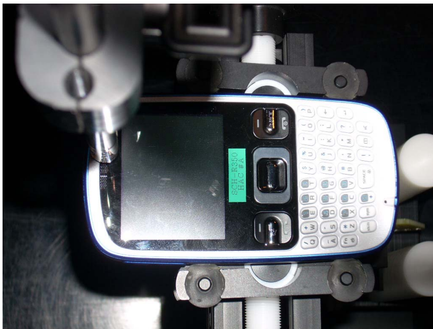
Figure 13-1 Test Setup for Wireless Device
