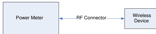
Figure 12-3 Power Measurement Setup
