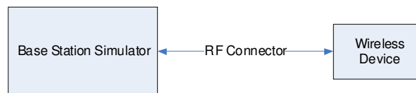
Figure 12-1 Power Measurement Setup
