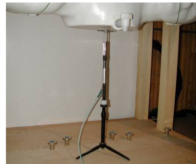
Figure 13-2 System Verification Setup Photo
