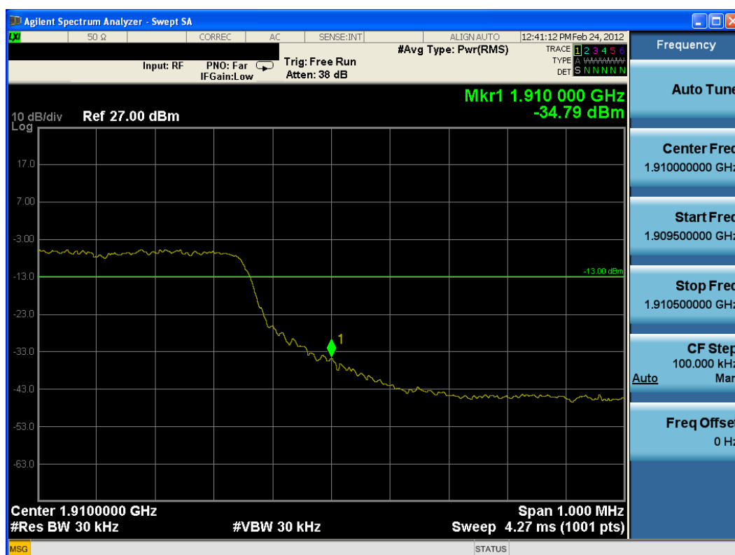
Plot 7-166. Upper Band Edge Plot (QPSK – RB Size 15)
