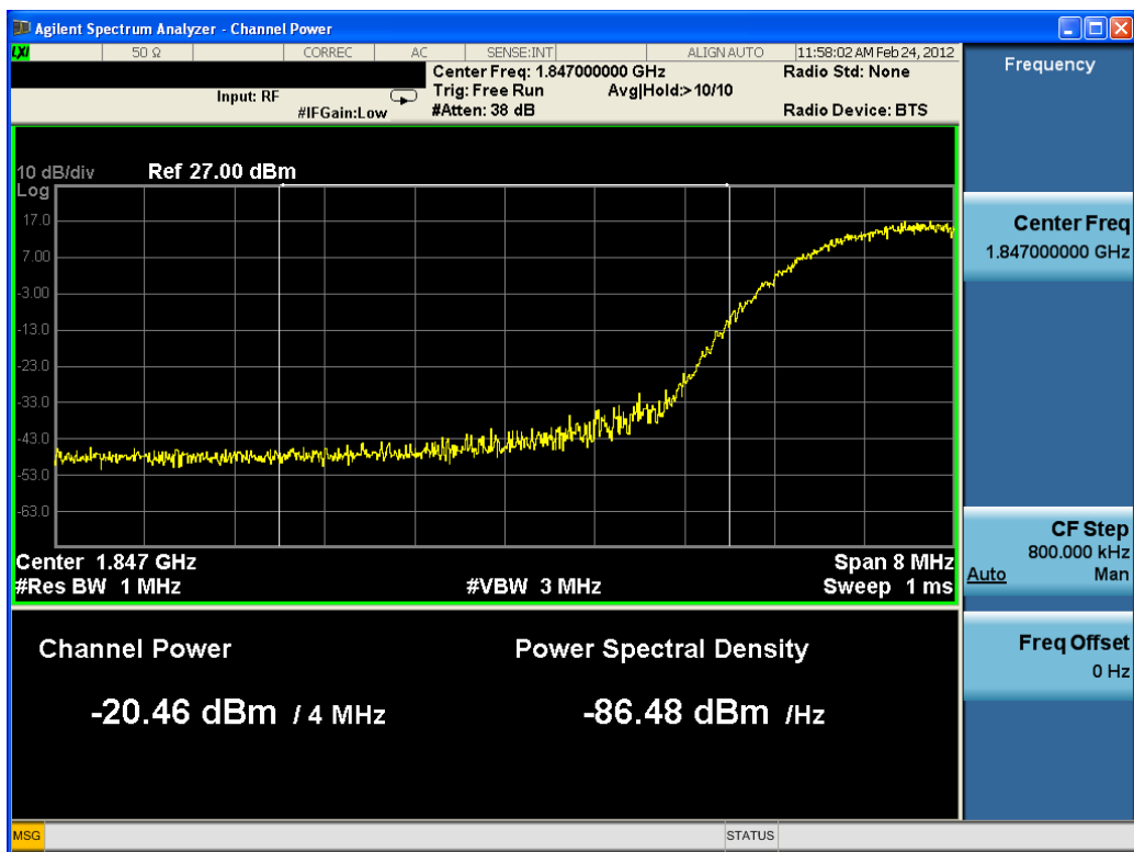
Plot 7-125. Lower Emission Mask (1845 – 1849MHz) Plot (16-QAM – RB Size 6)
