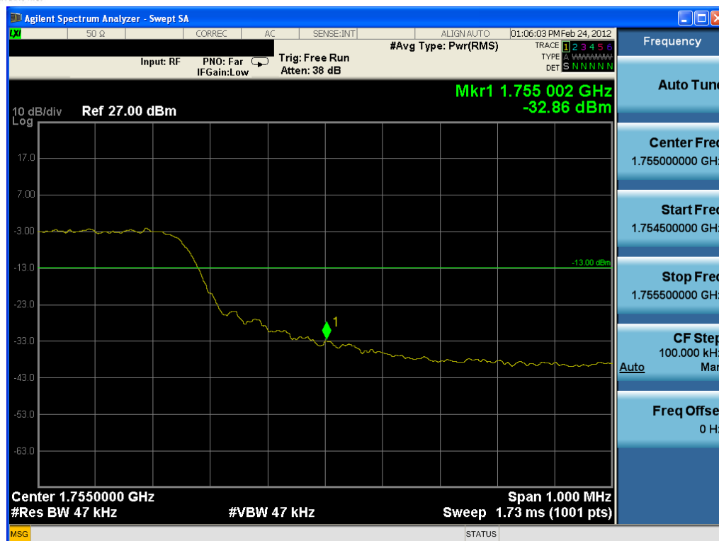
Plot 7-219. Upper Band Edge Plot (16-QAM – RB Size 25)
