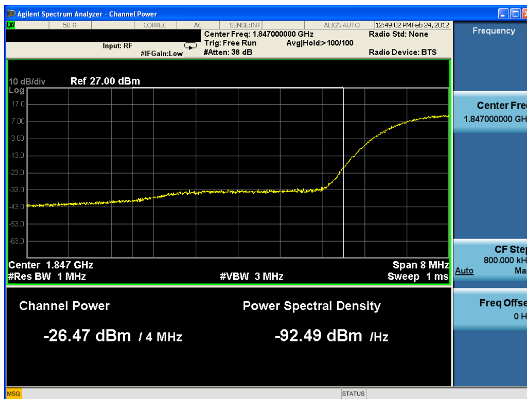
Plot 7-176. Lower Emission Mask (1845-1849MHz) Plot (QPSK – RB Size 25)
