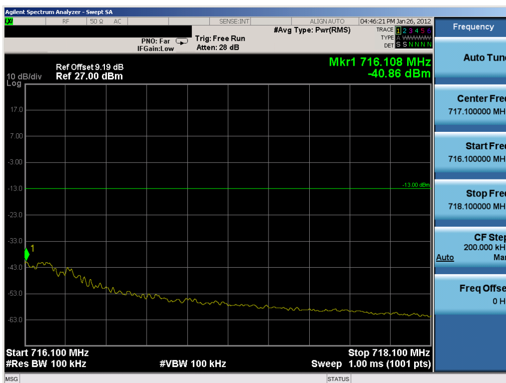
Plot 7-117. Upper Band Edge Plot (16QAM – RB Size 1, Offset 49)
