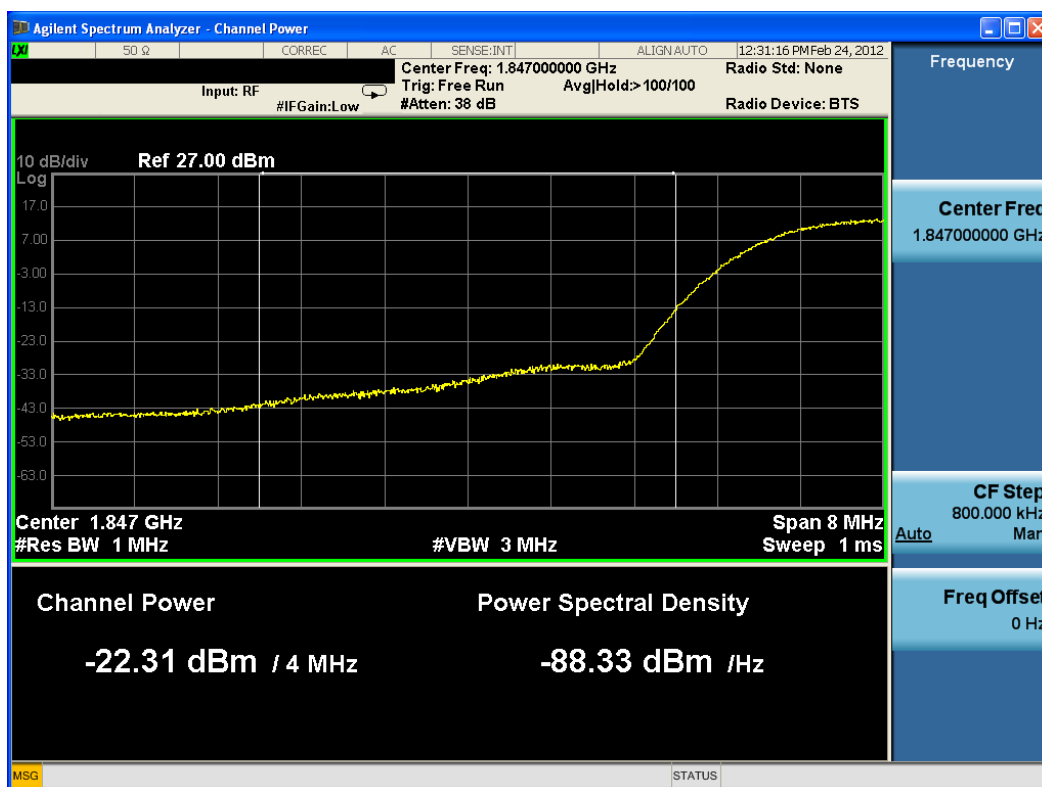
Plot 7-150. Lower Emission Mask (1845-1849 MHz) Plot (QPSK – RB Size 15)
