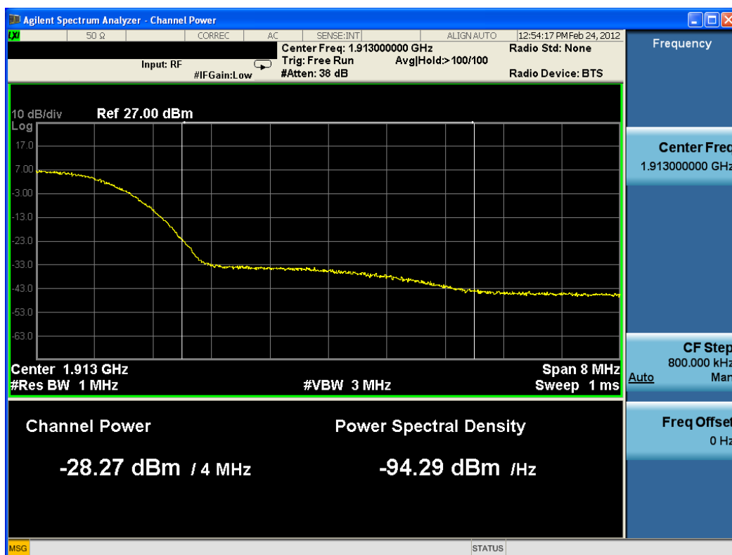
Plot 7-194. Upper Emission Mask (1911-1915 MHz) Plot (QPSK – RB Size 25)
