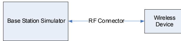
Figure 9-1 Power Measurement Setup
