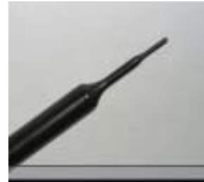
Figure 3.4 Probe Thick-Film Technique
