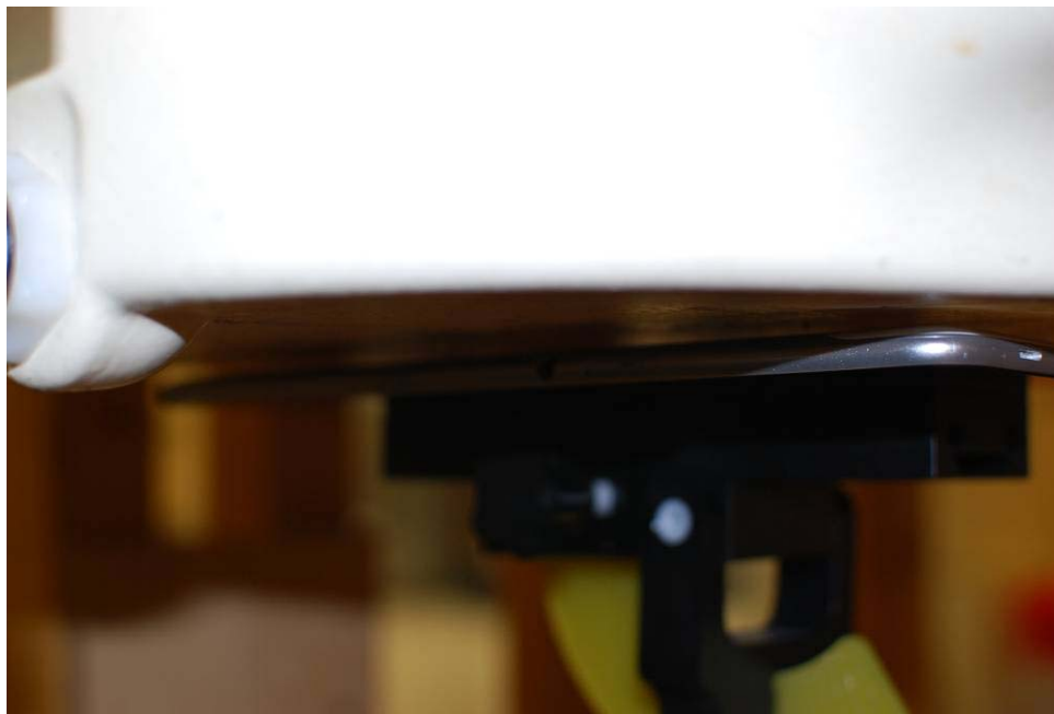
Figure 22-2 SAR Test Setup Photo 2: Back at 0.5 cm
