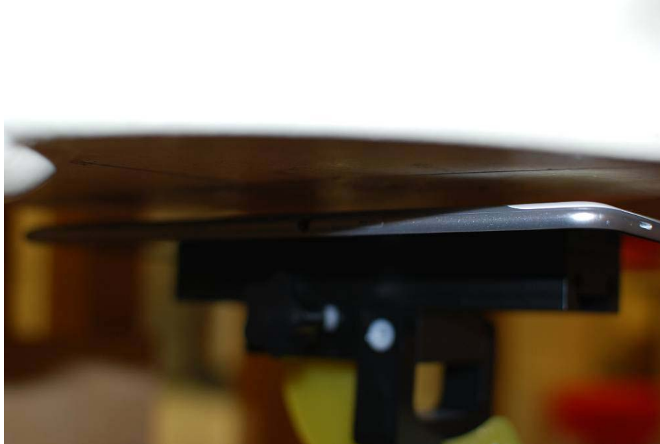
Figure 22-3 SAR Test Setup Photo 3: Back at 1.0 cm
