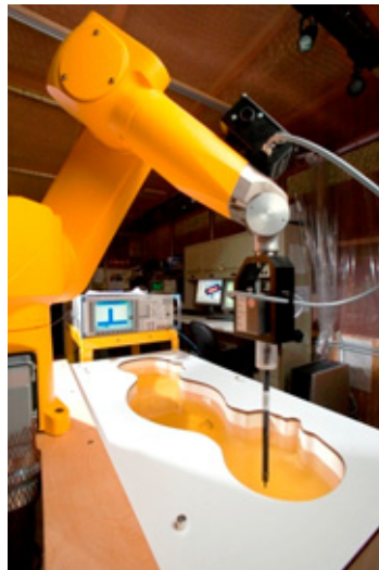
Figure 3-2 DASY4 SAR Measurement System
